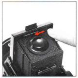
B. The magnifier is flipped into viewing position, by simply sliding the release lever in the arrow-indicated direction.
