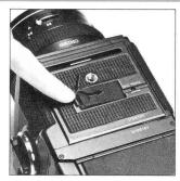
A. Depress the battery chamber button with your finger and, at the same time, move the battery chamber cover in the arrow-indicated direction. The cover will come off easily.
