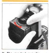
D. The standard magnifier supplied with the waist-level finder has a power of -1.50 diopters, which can be exchanged for others with powers of +1.50, +0.50, -0.50, -2.50, -3.50 and -4.50 diopters. These optional accessories should be purchased to suit the user's eyesight, if necessary.
