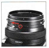
\* Except for time exposures, always shift the time exposure lever so that "A" is visible on the lens barrel and keep it locked with the setscrew to prevent accidental movement.
