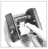
B. Remove the film holder and, while preventing the loose film from unwinding, take out the take-up spool. Seal the exposed film and return it to its original box until development.
