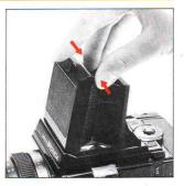
C. To close the focusing hood, first, push down the magnifier (if it is in viewing position). Next, press in both side frames, as illustrated, and, at the same time, press the front frame back towards the rear. The focusing hood will automatically he folded down.
