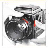
B. To detach the lens, the film winding crank must also be rotated to cock the lens shutter first. Then, press the lens release button down and, at the same time, rotate the lens in the clockwise direction until it makes a full stop, at which point it will be possible to detach the lens.
