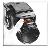
To attach the lens to the body, next, align the orange dots on the lens and body and then insert the lens fully into its mount. Rotate in the counterclockwise direction until it stops, with an audible click, which will indicate that it is securely locked.
