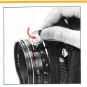
B. Next, cock the shutter with the film winding crank and then shift the time exposure lever to the left (looking from the body towards the lens) which will expose a red-colored "T" on the barrel. The shutter will stay open when the shutter release button is depressed in this condition.
