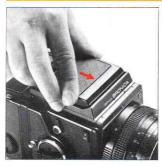
A. The finder can be interchanged, with other optional finders, to match shooting conditions to photographic conditions. To attach the finder, align the front end of the finder with the front end of the finder frame on top of the camera body, as shown. Then, gently lower the finder and, when well-seated, slide forward until it locks.
